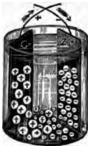
FIG. 16. Atoms of hydrogen marked + collected upon — copper, atoms of oxygen marked — set free at + zinc. Arrows show direction of current before polarization occurs.
